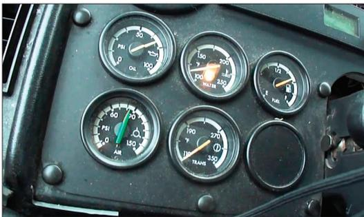
*“Airbrake build rate is acceptable”.*
