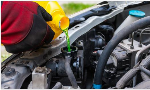
*“Coolant added to correct level”.*
